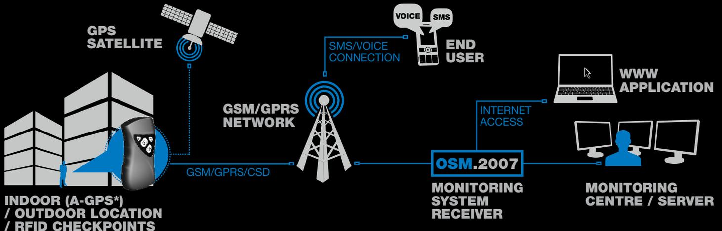
\* GPS users expect instant position information. With standard GPS this is sometimes not possible because at least four satellites must be identified, and their complete orbital position data, called Ephemeris, received.
